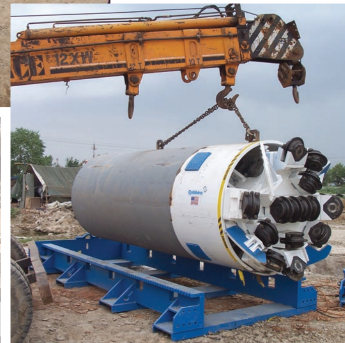
Below: The Robbins SBU utilised in Kota City is India's first-ever use of disc cutting heads.
